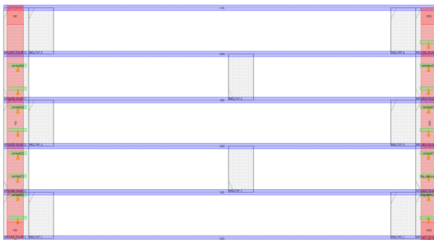
Figure 5.15 – An example of power plan and pin distribution for the Complementary-DE IP.
