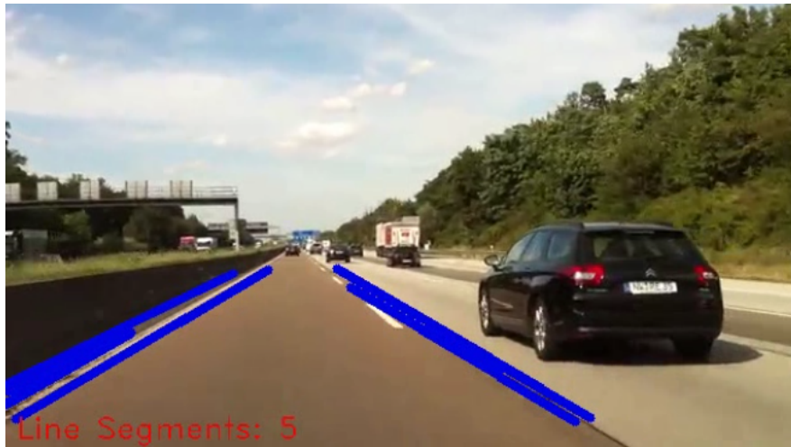
Figure 6.2 – Lane Detection - Processed Image.
