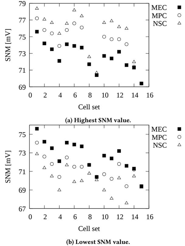
**Figure 7: Comparison between techniques lowest (a) and highest (b) SNM estimates at 250 mV supply voltage. X-axis corresponds to the "Ref" column of Table 2.**
