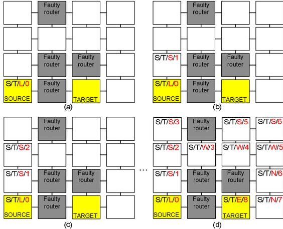
Figure 2 – Seek steps of the algorithm in a 4x4 mesh, with four faulty routers.
