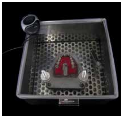
Figure 4 - Simulator submerged in warm water (50° C) controlled by a thermostat and a timer to allow tooth movement.
