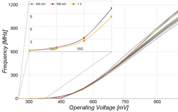
Fig. 3: Frequency vs. Operating Voltage for different Synthesis Voltage
