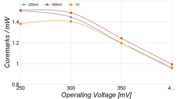
Fig. 6: Maximum Coremarks over Total Power vs. Operating Voltage for three different synthesis voltages: 250mV, 500mV and 1V
