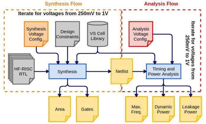
Fig. 2: Voltage scaling aware design and analysis flow.
