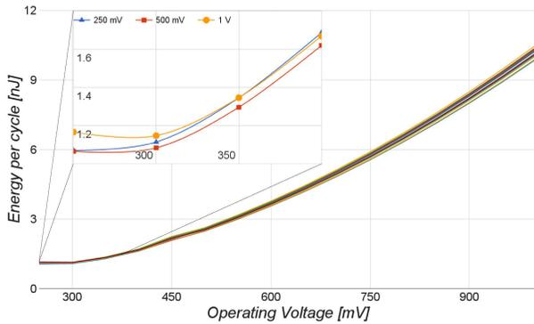
Fig. 4: Energy / Cycle vs. Operating Voltage for different Synthesis Voltage
