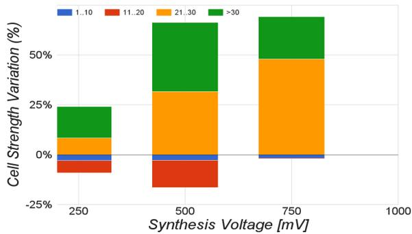
Fig. 8: Cell strength variation for 250mV, 500mV and 750mV synthesis compared to 1V.
