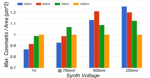
Fig. 7: Maximum Coremarks over Area vs. Synthesis for three different synthesis voltages: 250mV, 500mV and 1V
