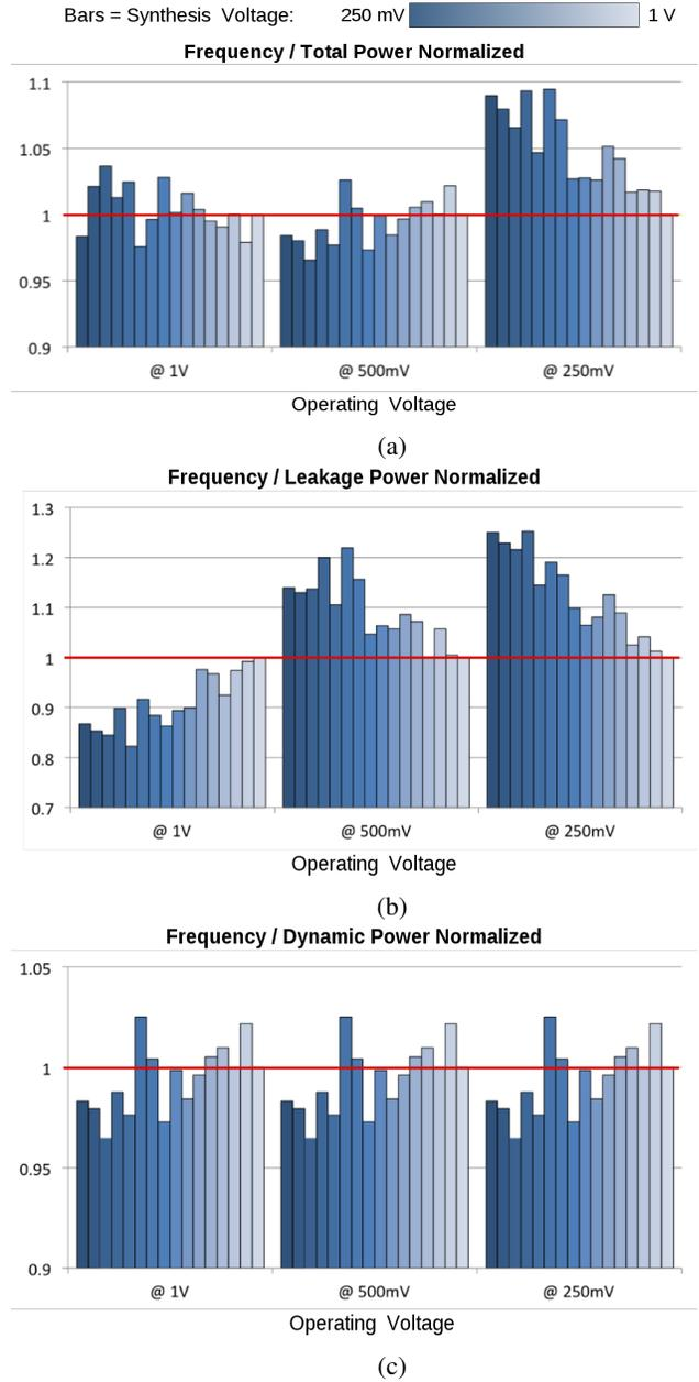
Fig. 5: Frequency over (a) Total Power, (b) Leakage Power and (c) Dynamic Power, all normalized to the 1V synthesis. In each is depicted three different operating voltages: @ 1V, @ 500mV and @ 250mV, and synthesis voltages varies from 250mV to 1V (left to right) for each.
