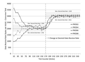
Fig. 7. Data receive rate adaptation at consumer task.
