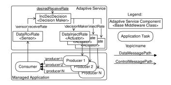
Fig. 6. Self-adaptive Prod-Cons application modelled using the middleware.
