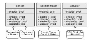
Fig. 2. Sensor, decision maker and actuator base classes and derivations.
