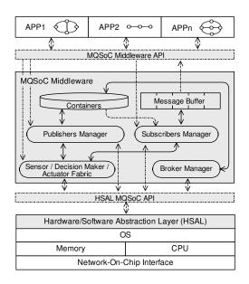
Fig. 1. Middleware structure and interfaces.
