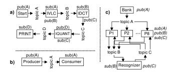
Fig. 4. Task graph of the a) MPEG, b) PROD-CONS, and c) DTW applications.
