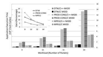
Fig. 5. Application execution time for C and C++ scenarios.
