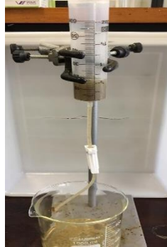
Figure 1. Drip in \text{CaCl}_2 solution to form capsules containing microorganisms.
