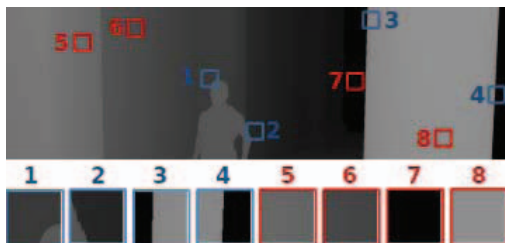
Fig. 1. Edges (1-4) and homogeneous regions (5-8) of a depth map.
