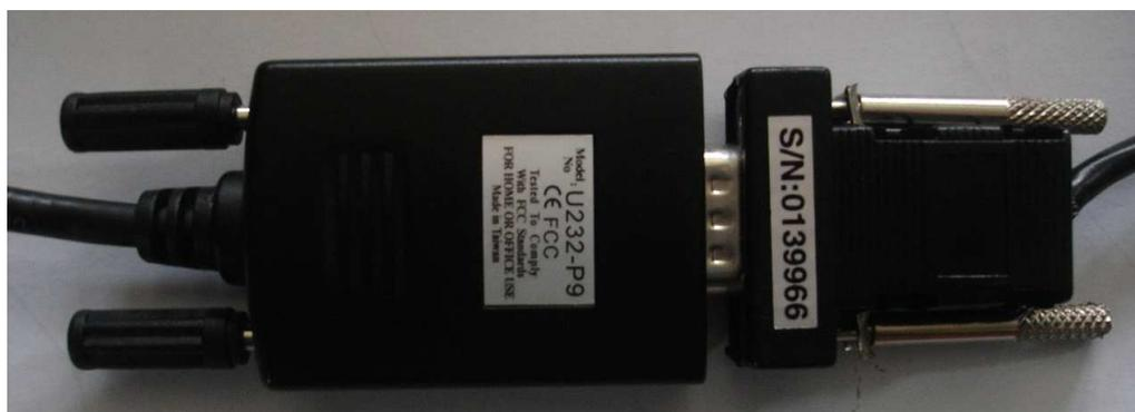
Figura 11 - Conversor RS485/232 - Conversor USB/232
