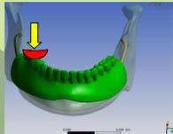
The models were loaded with a 100 N-axial vertical load applied on the right first molar, using a masticatory bolus simulation modeled as a rigid semi-sphere placed over the denture tooth (Daas et al., 2007).
