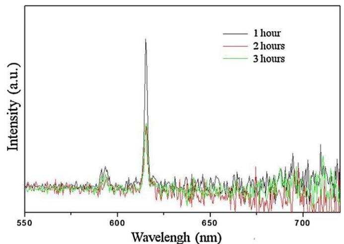
Fig. 5. Emission spectrum obtained in Europium-incorporated PLA films 1, 2 and 3 h after ethanol elution. a.u.: arbitrary units.
