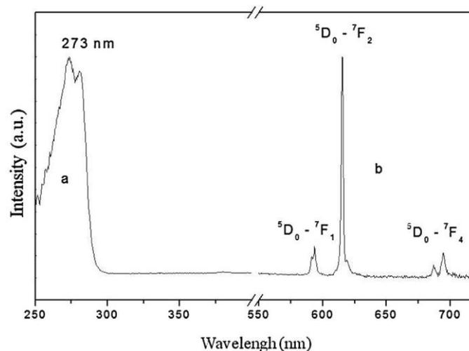
Fig. 4. Excitation (a) and emission (b) spectrum of Europium(III) complex after incorporation to PLA film.  ${}^5D_0 - {}^7F_1$ ,  ${}^5D_0 - {}^7F_2$  and  ${}^5D_0 - {}^7F_4$  represent the ion energy level related to electronic transitions occurring in Europium(III) compound. a.u.: arbitrary units.
