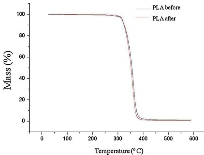
Fig. 3. Thermogravimetric curve of PLA film before and after contact with CHO-K1 cell. The temperature of thermal decomposition is between 300 and 400 °C.
