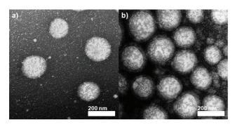
**Figure 1.** Transmission electron photomicrograph of the nanoemulsions DA at 150 k (b) and DB at 75 k (a).
