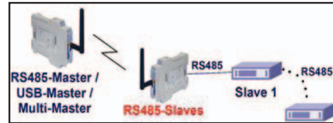
Figure 5. Operation Mode RS485-Slaves.
