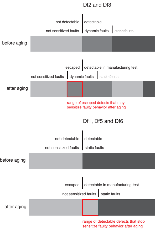
Fig. 13. Scheme for faulty behavior before and after aging.
