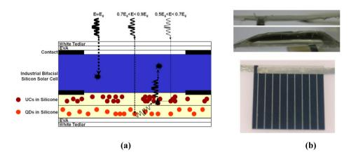
Fig. 4. (a) Encapsulation scheme: industrial BSSC laminated to UC and QDs in silicone. \* represents the generation of an electron-hole pair and ▲ the UC phenomena. (b) Pictures of the developed encapsulation: cross section with silicone+UC+QDs (above) and frontal view (below)
