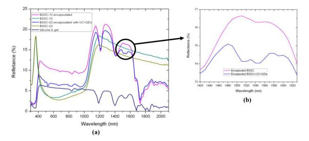
Figure 5. (a) Reflectance of the encapsulated BSSC with and without UC and QDs embedded in the silicone and (b) zoom of the reflectance in the range 1420 nm-1640 nm (<sup>4</sup>I<sub>13/2</sub> (<sup>4</sup>I<sub>15/2</sub> Er<sup>3+</sup> ion transitions).
