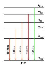
Fig. 3. Emissions of the Er<sup>3+</sup> doped materials under excitation around 1500 nm.
