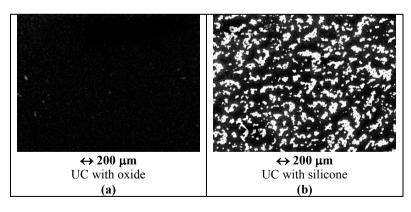
Figure 1. SEM pictures at a magnification of 95 commercial UCs increases attached in spin-on oxide (a) and silicone gel (b) [18].
