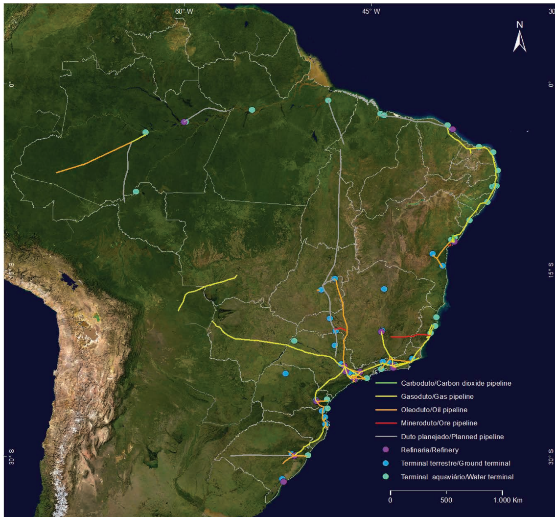
Figure 36: Current and planned pipeline network.
