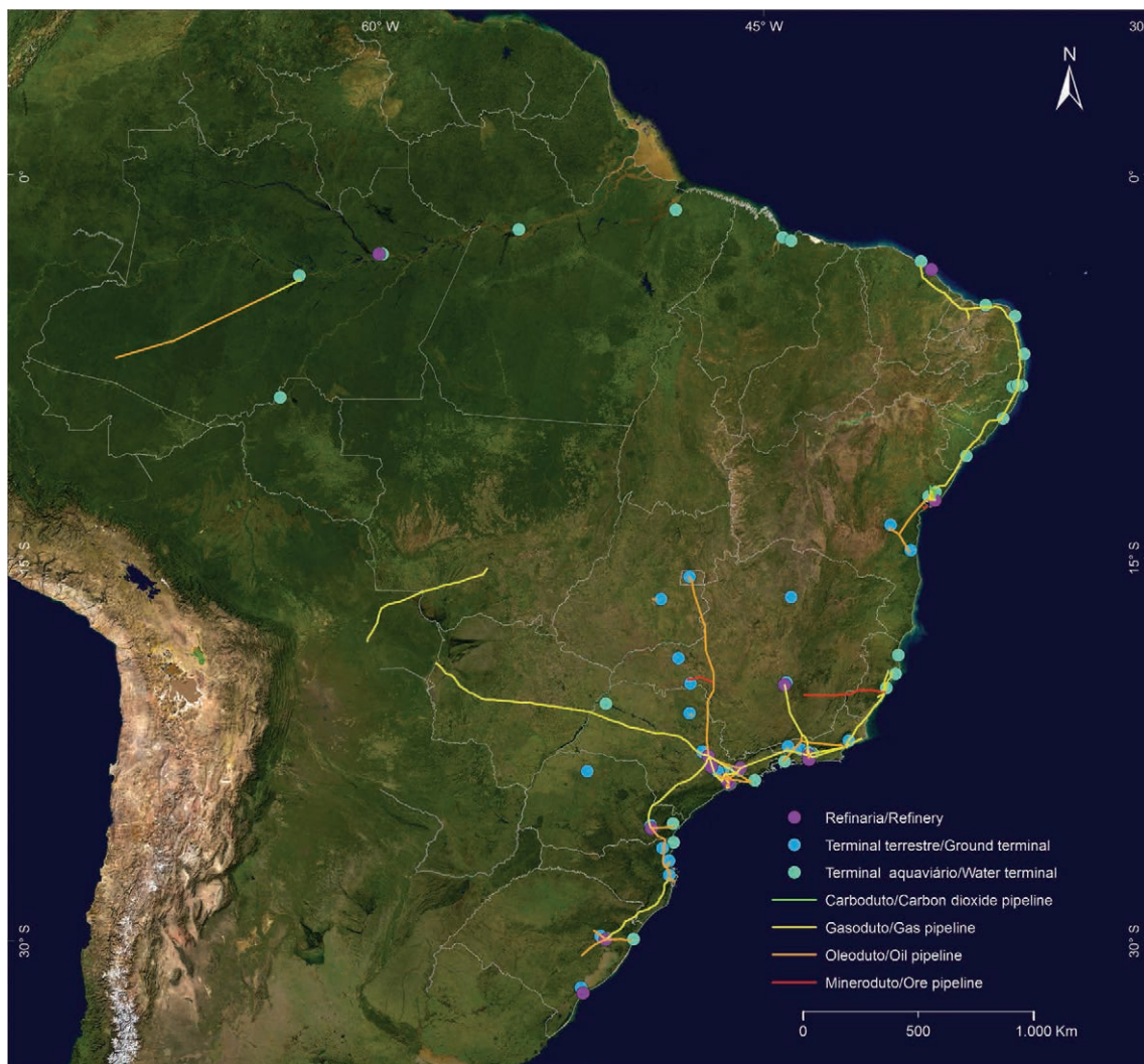
Figure 33: Pipeline network and terminals.
