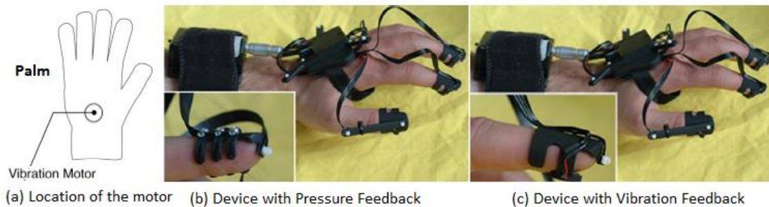
Figure 13 – Reception points for haptic feedback in (a) Niinimake et al. [19] and (b) (c) Moehring et al. [20].
