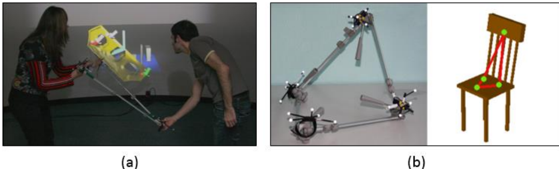
Figure 18 – (a) Example of a collaborative manipulation of a virtual car hood and (b) example of configuration of the RTD-4 for manipulating a virtual chair
