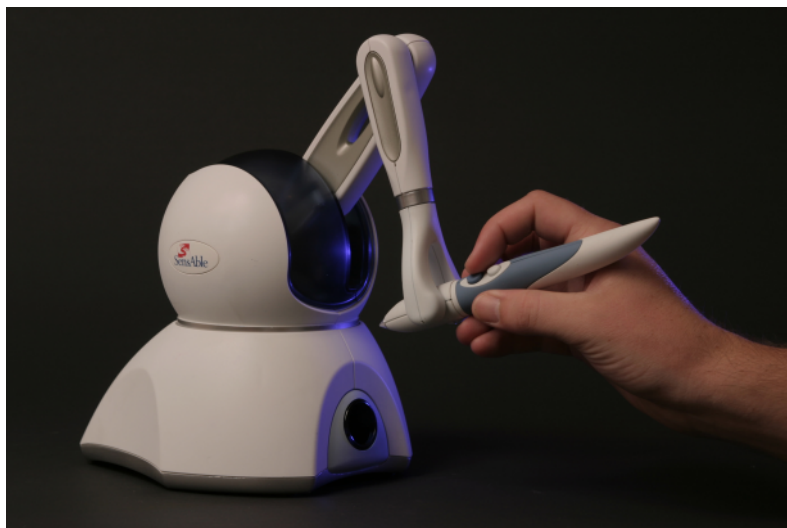
Figure 5: An example of a device that provides haptic feedback, known as Phantom Source: < http://www.sensable.com/haptic-phantom-omni.htm >.
