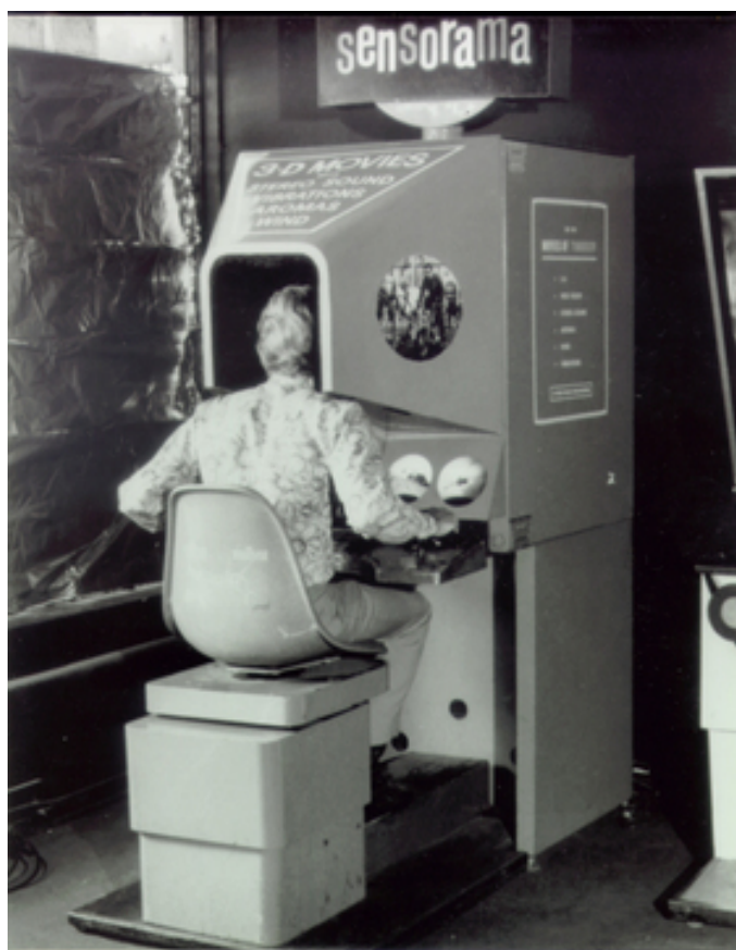
Figure 1: The first VR-like experiment, known as Sensorama, which simulated a motorcycle ride
