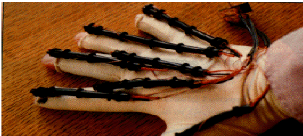
Figure 3: Data-glove, which users light sensors to calculate fingers' movements Source: < http://www.inf.pucrs.br/~pinho >.
