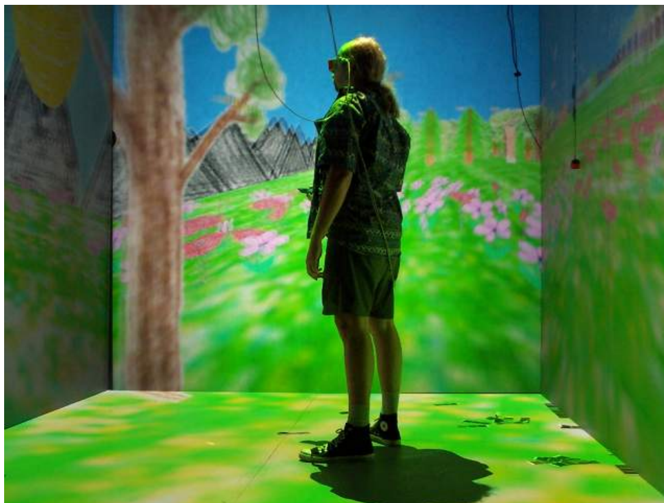
Figure 4: A user in a CAVE, which uses projection displays to surround the user and increase immersion
