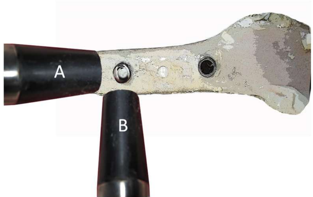
Fig 3. Schematic illustration of the implant stability quotient (ISQ) measurement in 2 directions: (A) disto-proximal and (B) antero-posterior.
