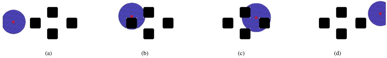
Fig. 5. Snapshots from experiment B , simulated with BioClouds. (a) A cloud heads towards an obstacle. (b) The cloud avoids the obstacle and increases its perception radius. (c) The cloud avoids another obstacle. (d) The cloud moves towards the goal and returns to its original size.
