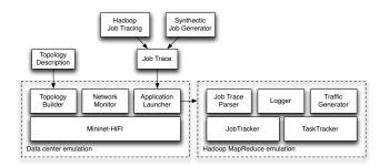
Fig. 1. Block diagram showing MRemu architecture.
