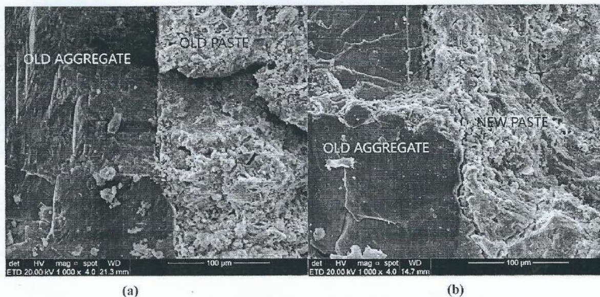
Fig. 17. SEM concrete containing 100% recycled aggregate and old paste (a), 100% recycled aggregate and new paste (b).
