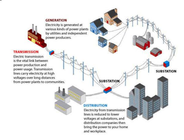
Figure 2.1 – Generation, Transmission and Distribution Grid Structure within the Power Industry [41]
