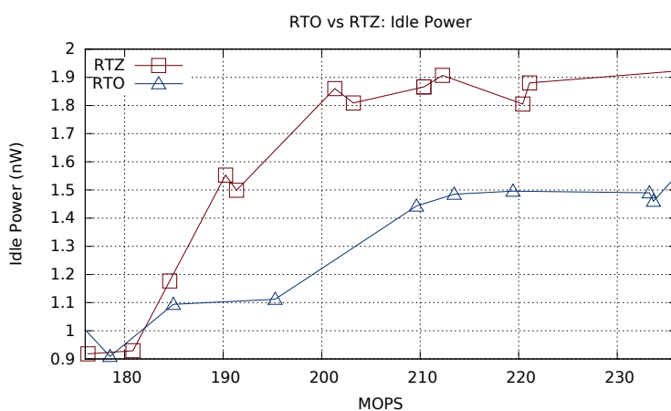
Figure 5.12 – Total power of the designs while at reset/set and idle states. Adapted from [MPC14].
