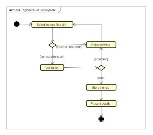
Figure 4.7 – User Engineer rule deployment activity diagram
