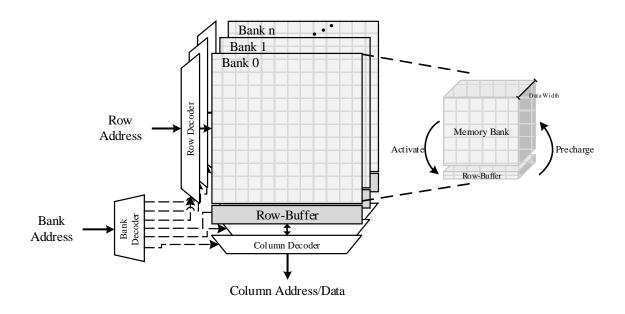
Figure 2.3: Internal DRAM structure. Source: created by the author.
