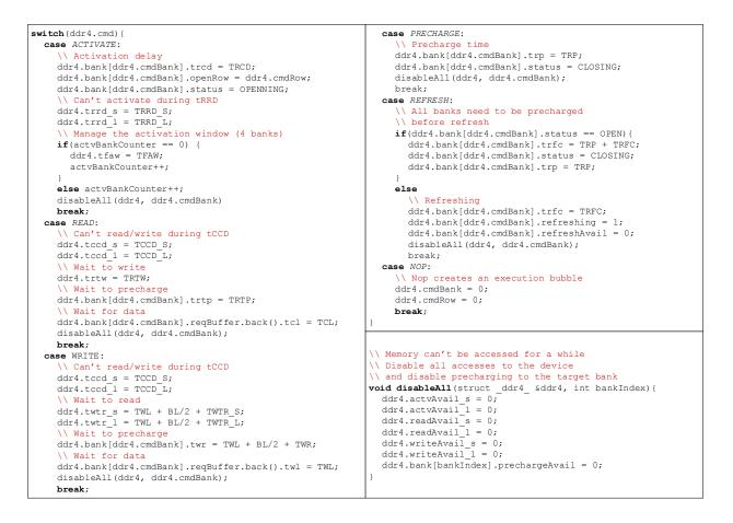
Figure 4.14: Pseudo-code for the command decoding logic. Source: created by the author.
