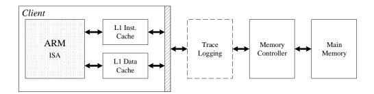
**Figure 5.1:** System architecture as created by Gem5. The dashed outline box represents the trace extraction module. Source: created by the author.
