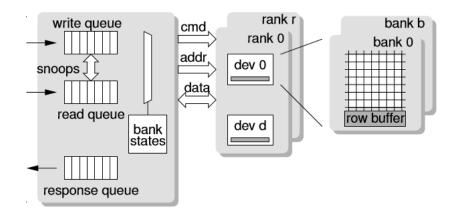
Figure 3.12: Hansson's read over write scheduling mechanism. Source: extracted from [H<sup>+</sup>14].
