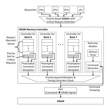
Figure 3.16: Structure of the priority-based controller proposed by H. Kim et al. (2015). Source: extracted from [K<sup>+</sup>15].
