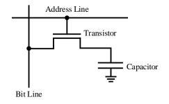
Figure 2.4: Internal DRAM cell structure (1T1C). Source: created by the author.
