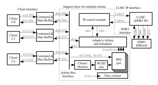
Figure 3.15: Block diagram of Bonatto's adaptive memory controller. Source: extracted from [BNP+14].
