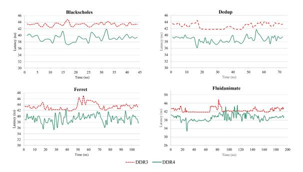
**Figure 5.4:** Latency comparison between DDR3-1333 and DDR4-2400 using 1.5GHz processors and the proposed simulator. Source: created by the author.
