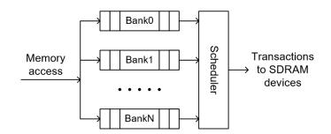
Figure 3.9: FCFS (bank-in-order) scheduling mechanism. Source: extracted from [Sha06].
