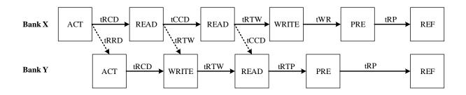
Figure 2.6: Timing dependencies between commands and banks. Dashed lines indicate inter-bank dependencies. Source: created by the author.
