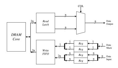
Figure 2.5: Input and output of a 2n prefetch architecture. Source: created by the author.
