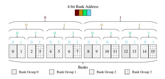
**Figure 4.3:** Mapping position of a 16-bank DDR4 in a 4-bit register considering four bank-groups interleaved. Source: created by the author.
