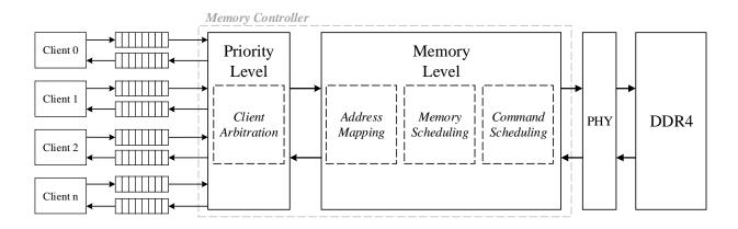
**Figure 4.1:** Proposed structure of the two-level memory controller: Priority Level and Memory Level. Source: created by the author.
