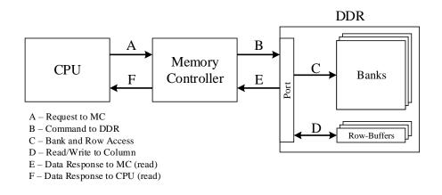
Figure 3.2: Data transference steps between CPU and DDR SDRAM. Source: adapted from [Bon14].
