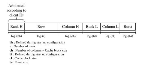
**Figure 4.10:** Proposed address mapping scheme considering a single channel and a single rank. The size in bits of each field is calculated through  $\log_2(x)$ , being x a variable dependent on controller configurations or memory module characteristics. Source: created by the author.
