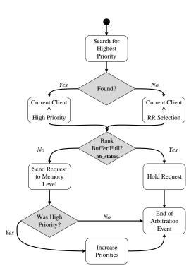
Figure 4.8: Client manager logic represented as a flow-chart. Source: created by the author.
