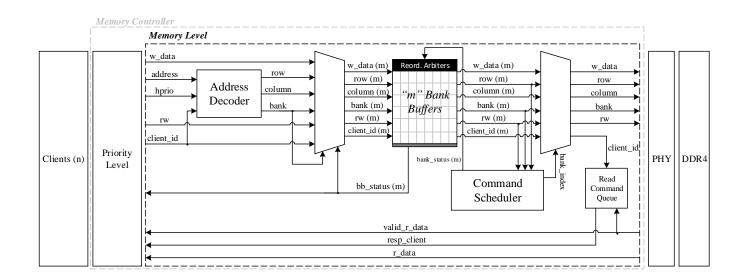
**Figure 4.9:** Block diagram of the *memory level*. The address decoder holds the mapping table and implements the bank privatization technique. The bank buffers store the memory requests and the reordering arbiters schedule requests using the proposed reordering algorithm. The command scheduler schedule commands considering bank-group constraints. Source: created by the author.
