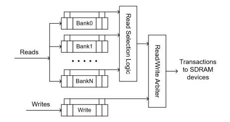
Figure 3.13: Intel out of order scheduling structure. Source: extracted from [Sha06].
