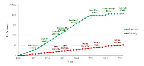
**Figure 1.1:** Performance evolution for processors and DRAMs. The memory frequencies presented in the labels of this plot consider data-bus frequencies. Memory internal clock frequencies are considerably smaller, therefore, explaining the *performance gap* [Jed16b]. Source: data extracted from [Car02][Li16][Mic16c].
