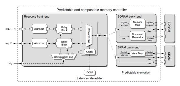
**Figure 3.14:** Predictable and composable memory controller divided into front-end and back-end parts. Source: extracted from [AG11].
