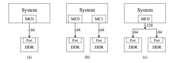
**Figure 3.1:** System configurations: (a) Single-channel (b) Dual-channel and (c) High-bandwidth 128-bit channel. Source: adapted from [Bon14].
