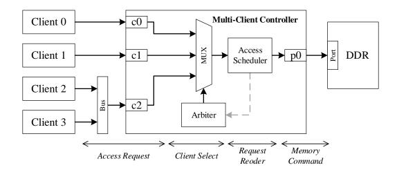
Figure 3.3: Illustration of a multi-client architecture with the request steps to memory access. Source: created by the author.
