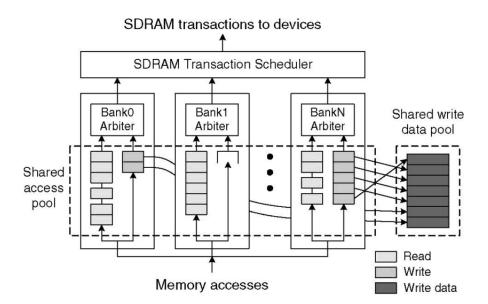
Figure 3.11: Burst reordering scheduling mechanism. Source: extracted from [SD07].
