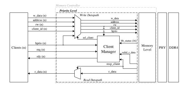
**Figure 4.6:** Block diagram of the *priority level*. The client manager implements the priority algorithm, the *n* clients are connected in parallel, and the write and read datapaths transfer data from e to clients, respectively. Source: created by the author.
