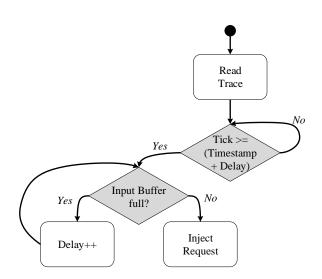
Figure 4.7: Diagram for the trace input logic. Source: created by the author.
