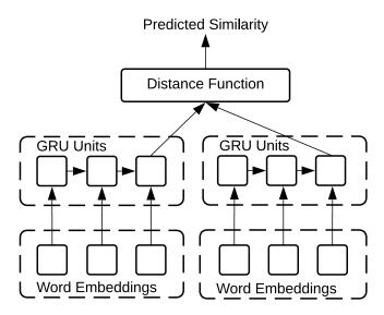
Fig. 1. Diagram ilustrating our siamese neural network defined, combining two recurrent neural network. The siamese network receives a sequence of word embeddings of the words contained in the input sentences, encodes into a sentence vector and learns a distance function to measure similarity.
