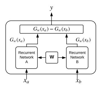
Fig. 3. Diagram illustrating weight structure W shared between two networks, predicting y through a metric learning given two inputs  $x_a$  and  $x_b$ , which is applied a  $G_w$  function.
