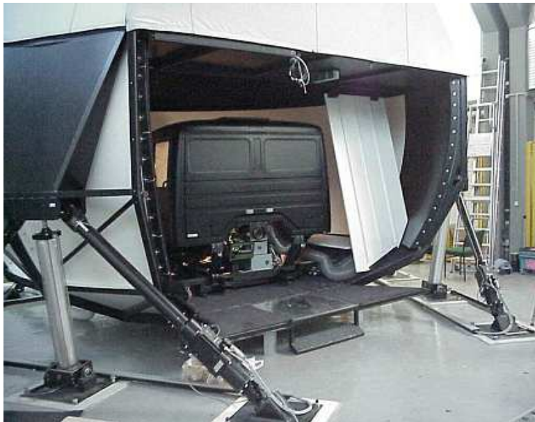
Figura 4 - Truck Driver Training Simulator
