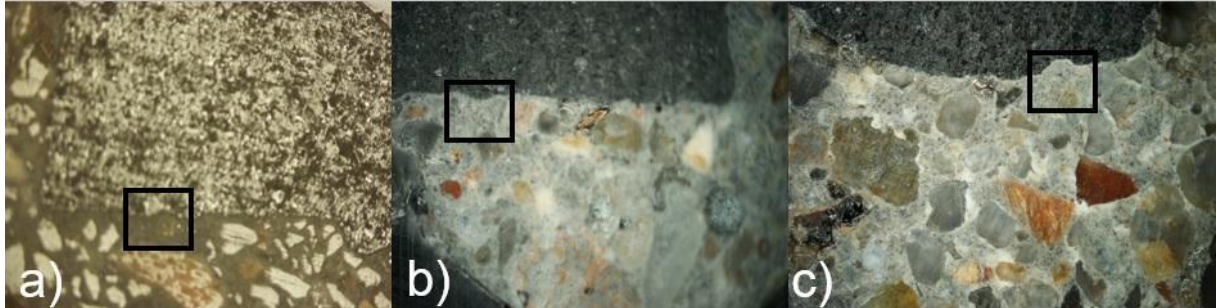
Figure 7: Optical microscopy images of concrete ITZs ( w/b = 0.35 ): (a) C3-SF0-NS0, (b) C3-SF10-NS0, (c) C3-SF0-NS3
