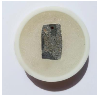
Figure 1: Sample of the prepared concrete for nanoindentation analysis
