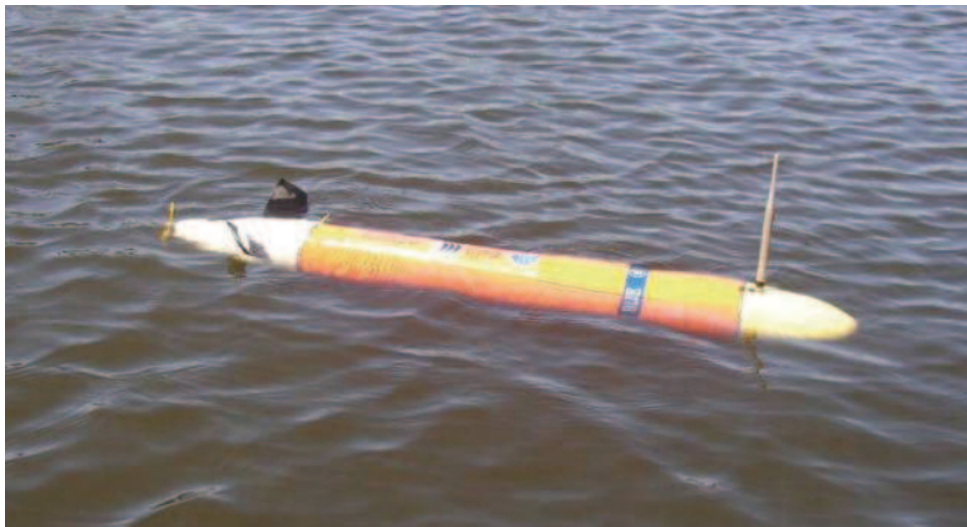
Figure 1: Light Autonomous Underwater Vehicle (LAUV) design and built at University of Porto.
