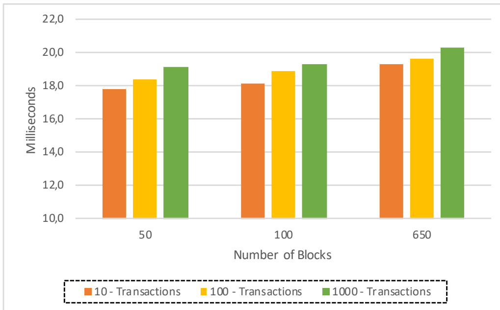
Figure 6.5 – Required time in an RSI to add a new block to the blockchain.
