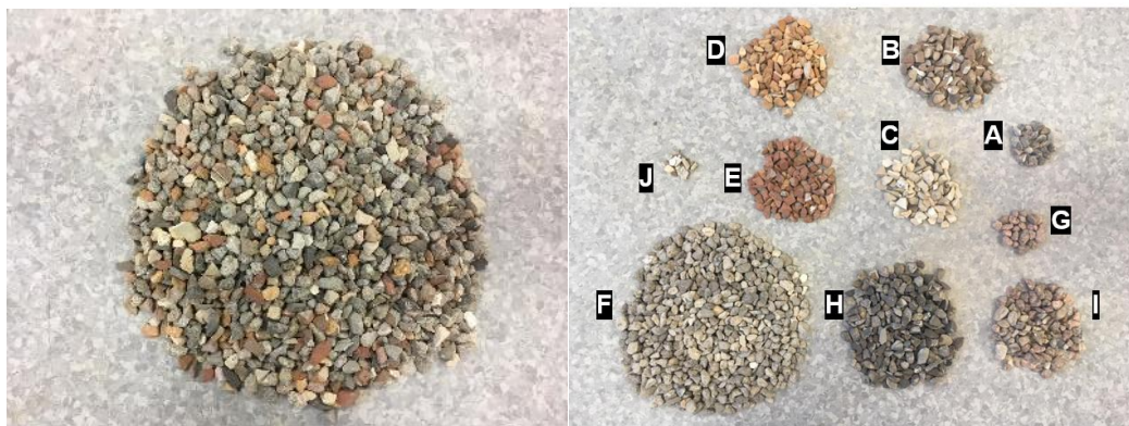
Figure 3: Crushed and mixed residue before (a) and after (b) manual separation.
