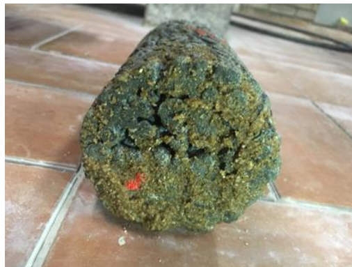
28 29 Figure 6: Cylindrical specimen after clogging test.
