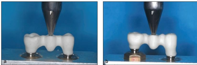
**Fig 1** Images of the three-unit CAD/CAM monolithic zirconium oxide FPD positioned in the universal testing machine for load application at the central fossa of the pontic. (a) Control group. (b) Test group.
