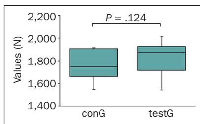
**Fig 2** Box plot of the values measured in the quasi-static test. The statistical analysis showed no difference between the groups. conG = control group; testG = test group.
