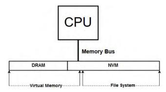
FIGURE 7. Target architecture - single address space model.
