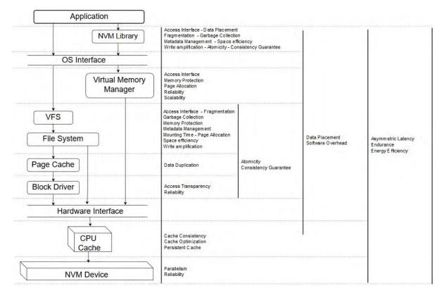
FIGURE 4. Diagram connecting the challenges identified with the respective architecture levels that address them.
