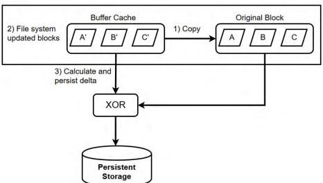
FIGURE 3. MRAMFS method to capture the delta between original and modified versions of a block [68].
