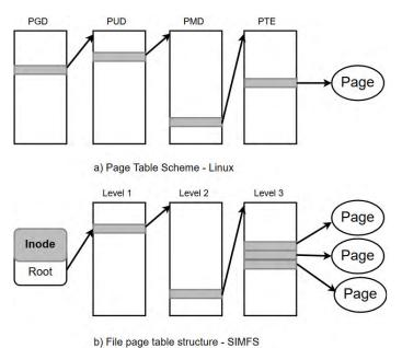
FIGURE 5. SIMFS index structure [119]. (a) Basic OS page hierarchical page table structure, (b) SIMFS file virtual address space index structure.
