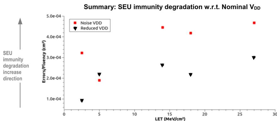
Fig. 9. Difference of the SEU immunity measurements for the “10.38% injected noise” and “continuous 1.34 V reduced  $V_{DD}$ ” operating conditions, with respect to the FPGA SEU immunity measured at nominal  $V_{DD}$ .
