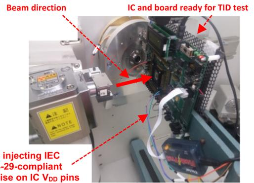
Fig. 5. Combined TID and conducted EMI test based on X-ray diffractometer equipment and noise injected directly on the V<sub>DD</sub> input power pin of the IC.
