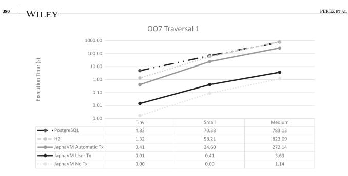
FIGURE 9 Comparison of execution times for traversal 1 (seconds, logarithmic scale)
