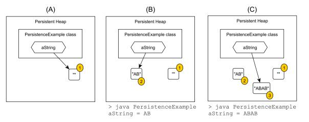
**FIGURE 2** Example of persistence by class attribute. A, After persistence example class loading; B, After first execution of main(); C, After second execution of main() [Colour figure can be viewed at wileyonlinelibrary.com]
