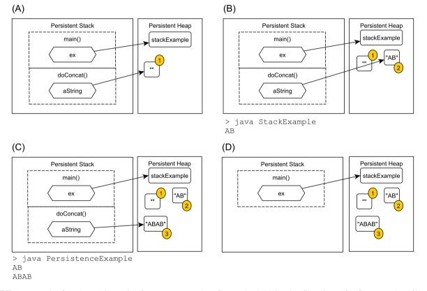
**FIGURE 5** Example of persistence by stack reference. A, Execution after a string initialization (line 4); B, After first execution of loop (line 5); C, After second execution of loop (line 5); D, After method doConcat() finishes [Colour figure can be viewed at wileyonlinelibrary.com]
