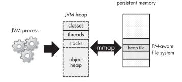
**FIGURE 6** Persistent memory hosting an in-memory file system, which contains a persistent heap file
