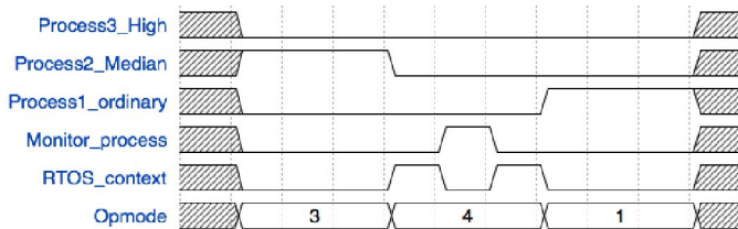
Fig. 4. Process switching time: switching between two application process and the Monitor process.
