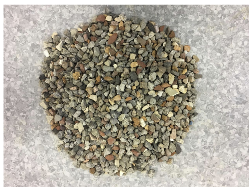
Fig. 3. Crushed and mixed residue before (a) and after (b) manual separation.
