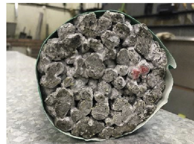
Fig. 5. (a) Scheme of the permeability test equipment (adapted from Lamb, 2014); (b): Specimen jacketed by the latex membrane.
