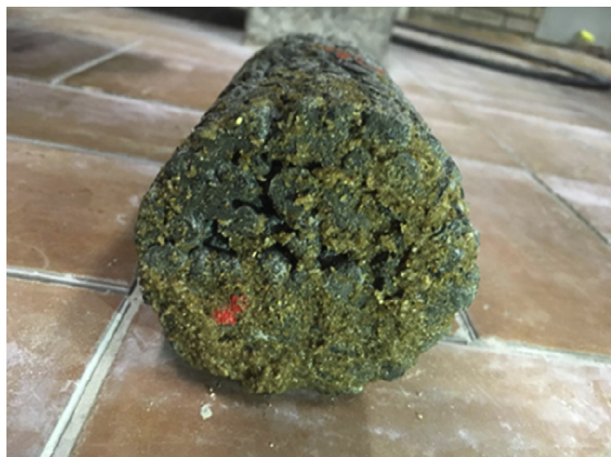
Fig. 6. Cylindrical specimen after clogging test.
