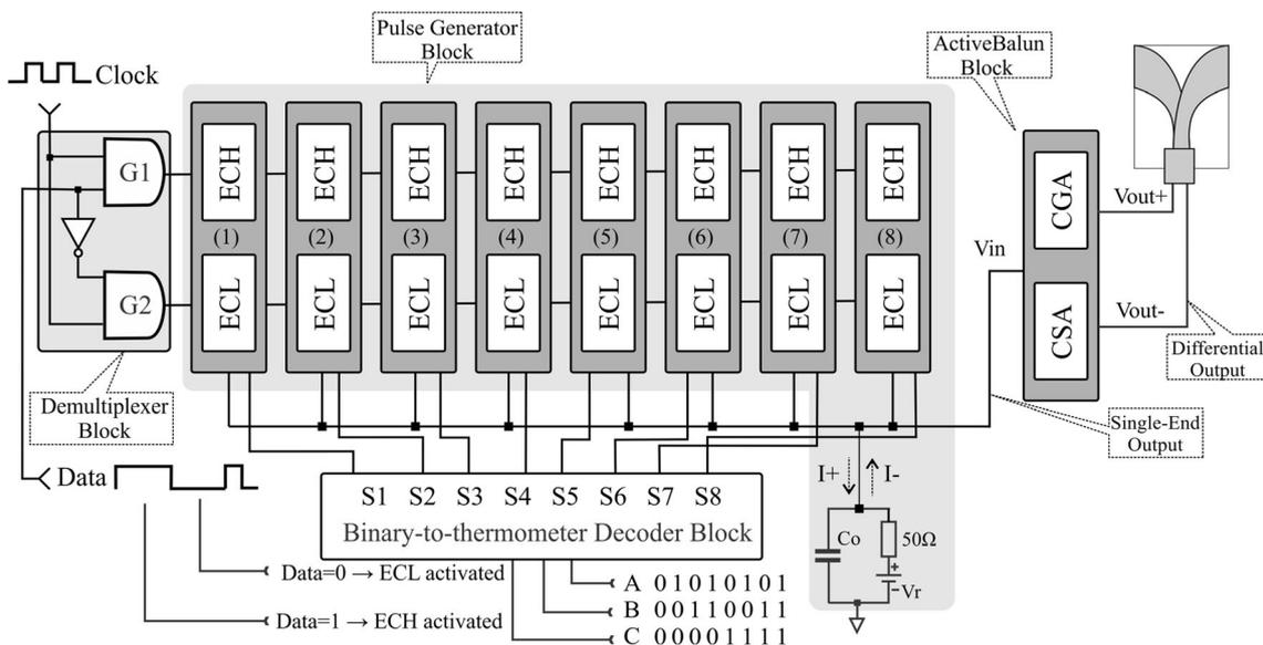
**Fig. 3** The detailed architecture of the implemented IR-UWB transmitter highlights the four main constituent blocks: demultiplexer, pulse generator, binary-to-thermometer decoder, and active balun
