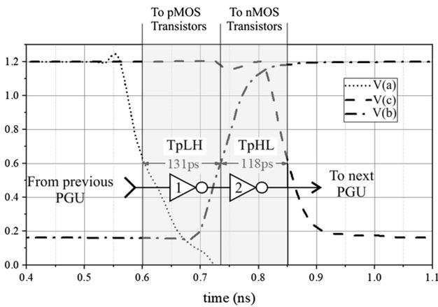
Fig. 10 Waveforms of voltages  $V_a$ ,  $V_b$ , and  $V_c$  of the delay circuit, showing phase differences
