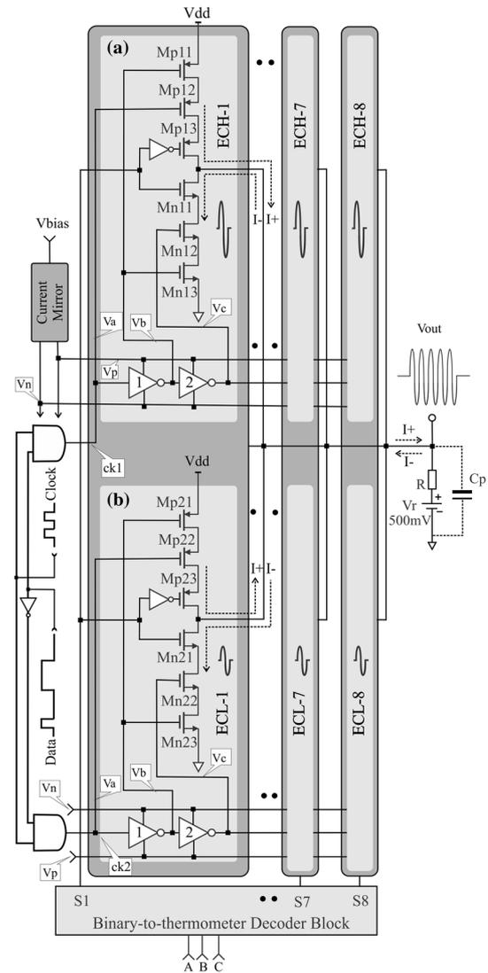
**Fig. 5** Diagram of the pulse generator with eight pulse generator units (PGU) using pulse amplitude modulation (PAM) scheme. The PGU-1 is presented in detail: **a** shows the edge combiner high (ECH-1), and **b** shows the edge combiner low (ECL-1)
