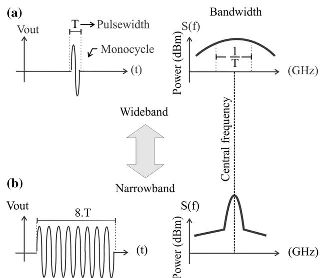
**Fig. 2** Waveforms and power spectral density of pulses with different monocycles per pulse: **a** a single-monocycle pulse and a wideband spectrum; **b** an eight-monocycle pulse and a narrowband spectrum
