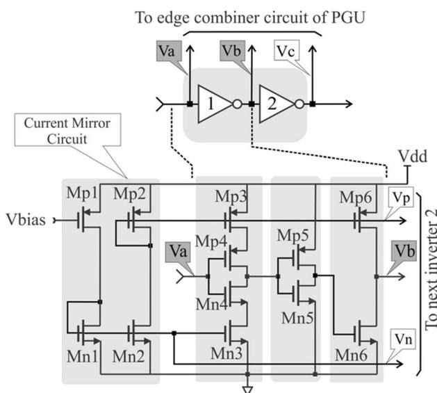
**Fig. 6** Schematics of the delay circuit
