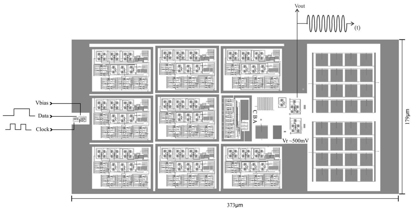
**Fig. 8** Complete layout of the proposed transmitter, without PADS
