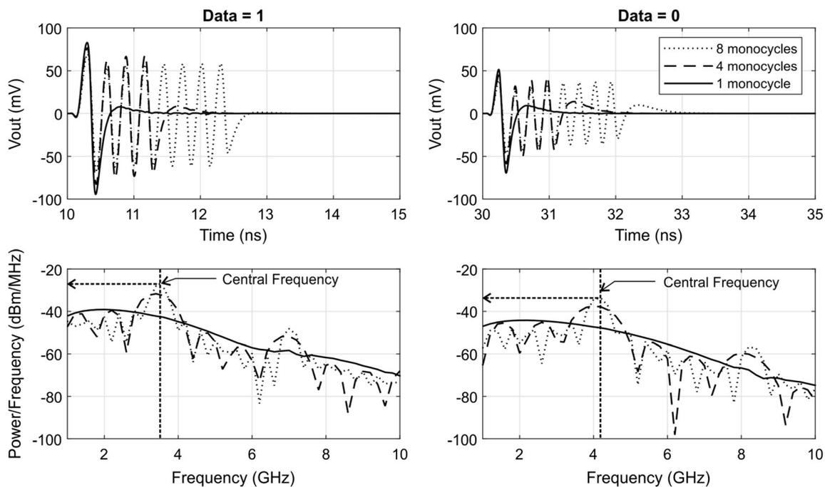
**Fig. 9** Power spectrum density (PSD) for  $Data = 0$  and  $Data = 1$ , simulated for 1, 4, and 8 monocycles. Top graphs show the output voltages, while the bottom graphs show their corresponding PSD.
