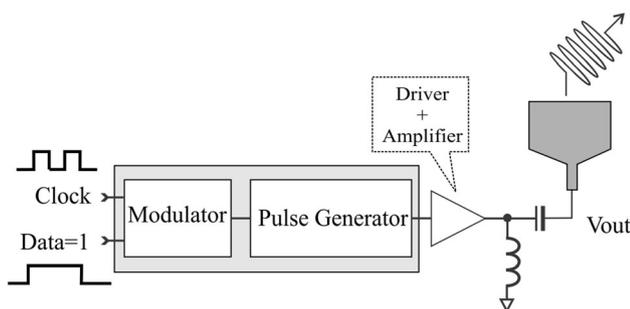
**Fig. 1** A generic block diagram of an IR-UWB transmitter comprising four building blocks: a modulator, a pulse generator, an amplifier, and an output driver
