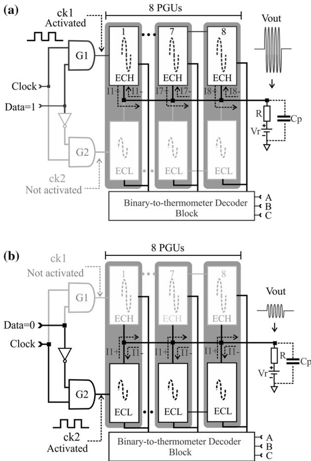
**Fig. 4** The operation mode of the pulse generator: **a** when  $Data = 1$ ,  $ck1$  and ECH are activated; **b** when  $Data = 0$ ,  $ck2$  and ECL are activated
