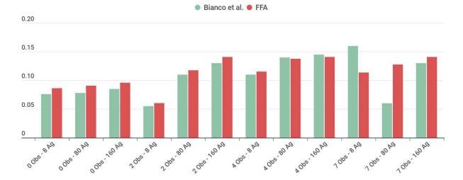
Fig. 4. Comparison of relative error in position (m) between the model presented by Bianco et al. [12] and our proposed FFA method. Values presented are an average between five executions. The value of a single execution is defined by the average Dif of all agents in the simulation, as defined by Equation 2. The number of frames affected by the FFA for each scenario is described in Section IV-D.
