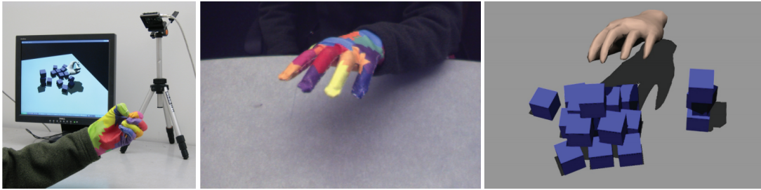
Figure 1.1 – "We describe a system that can reconstruct the pose of the hand from a single image of the hand wearing a multi-colored glove. We demonstrate our system as a user-input device for desktop virtual reality applications." Source: [46]
