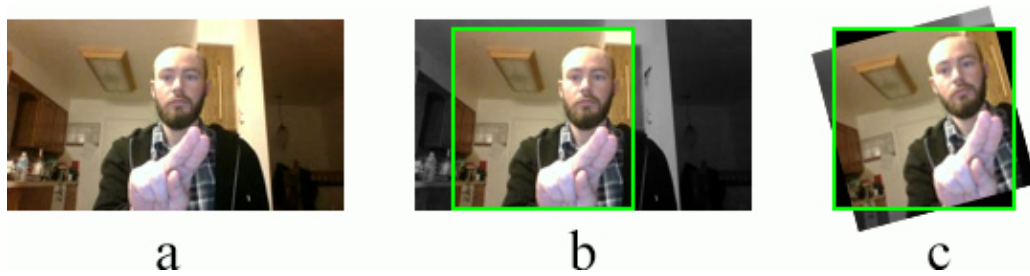
Figure 4.10 – Data Augmentation for the Jester Dataset. a) Original Image, b) "Randomly" cropped image and c) "Randomly" rotated Image
