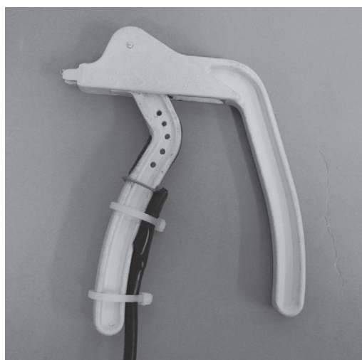
Figure 1 Polypropylene pliers with the five holes in the top one-third of the active arm lateral surface; strain gauges are bonded to the anterior and posterior active arm face of the pliers.
