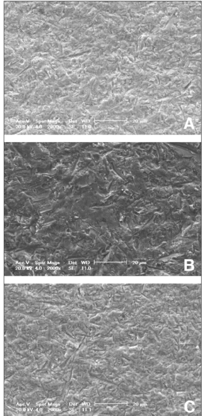
Figure 5. SEM of In-Ceram Alumina (a) Control (original magnification 2000x), (b) Airborne particle abrasion with 50- $\mu$ m aluminum oxide for 15 seconds (original magnification 2000x), (c) Etching with 9.5% hydrofluoric acid for two minutes (original magnification 2000x).
