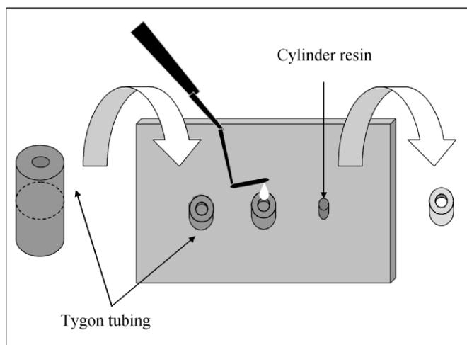
Figure 1. Scheme of the bonding procedure.
