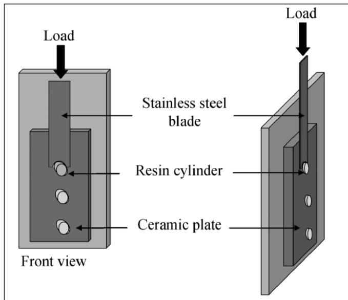
Figure 2. Schematic views of the micro-shear bond test.
