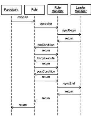
Fig. 13. Sequence diagram for the normal behaviour of a CAA.
