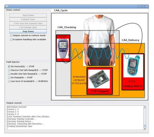
Fig. 24. Injecting a fault on the sensor.
