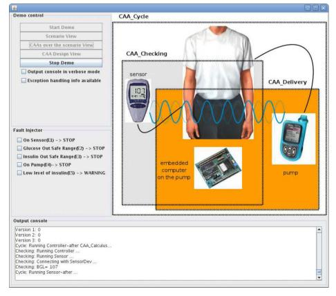
Fig. 23. The Fault-Tolerant Insulin Pump simulator.
