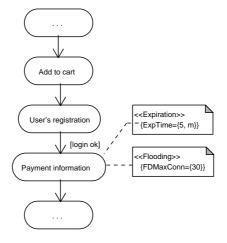
**Fig. 4.** Application of  $\ll$ Expiration $\gg$ and  $\ll$ Flooding $\gg$  stereotypes
