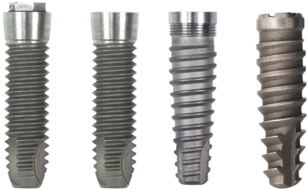
Fig. 1 Image of the implants used in the study: cylindrical external hexagon (3.30 mm), cylindrical internal hexagon (3.30 mm), conical internal hexagon (3.50 mm), and conical Morse taper (3.50 mm), respectively
