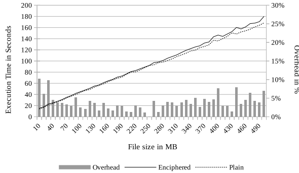
Fig. 7. Hadoop overhead by CFS: Word count running over different files sizes.
