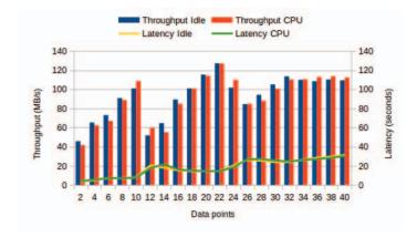
Fig. 3. Performance degradation in MB/s and latency using Stress-ng.
