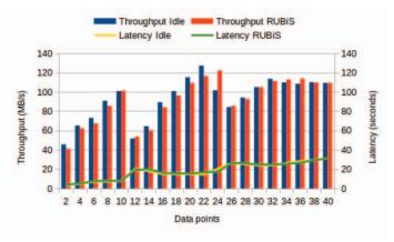
Fig. 7. Sample I/O Load Levels Versus Latency for RUBiS application.
