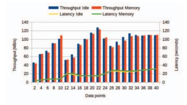
Fig. 4. Performance degradation in MB/s and latency using Stressapptest.
