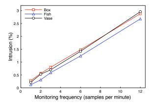
Fig. 6. CASViD Monitor's Intrusion with Different Sampling Frequencies.
